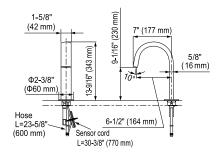
■Mounting deck thickness: 1/4" (5 mm) - 2" (50 mm)
